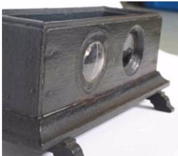
Figure 2b: Water Lenses I – Simple water lenses in the 17th century could have looked like these ones that consist of convex plate glasses made of hollow glass and flat sheets of glass, stuck with putty into wooden frames or boxes.
