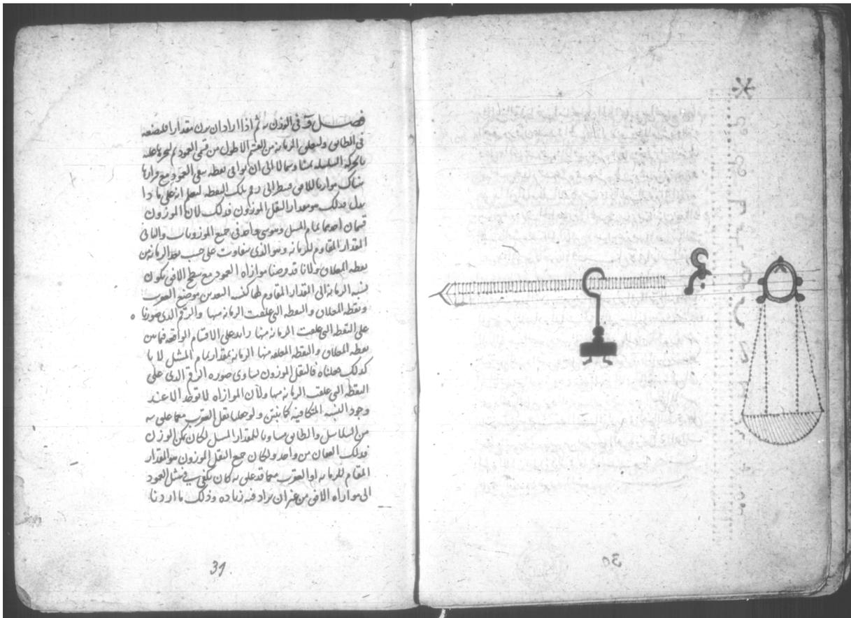
**Figure 8.** MANUSCRIPT PAGE OF BOOK II OF AL-KHAZINI’S “BOOK OF THE BALANCE OF WISDOM,” WRITTEN ABOUT 1120 A.D., WHICH CONTAINS A DETAILED DESCRIPTION OF THE PROCEDURE TO CONSTRUCT THE SCALES OF A STEELYARD (ST. PETERSBURG, MS. KHANIKOFF, FOLIO PAGE 30 VERSO)
