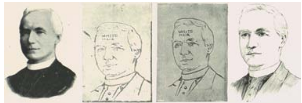
Fig. 4: Stages of transmission by telediagraph from Washington, DC to the offices of the New York Herald . As the telediagraph could not transmit color, the sending party inscribed "white hair" on the image for the benefit of the receiver. Charles Cook, "Pictures by Telegraph," Pearson's 3:4 (1900).
