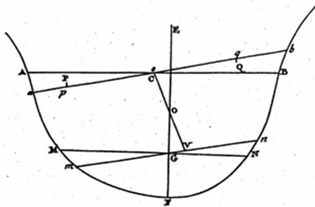
Fig. 6: Euler's Centroid Shift in Inclined Cross Section (from [54])
