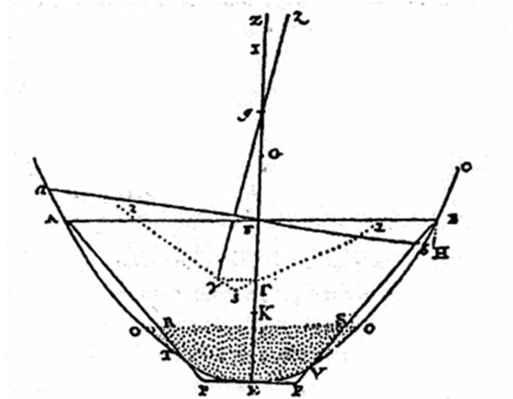
Fig. 5: Bouguer's Derivation of the Metacenter (from [53])
