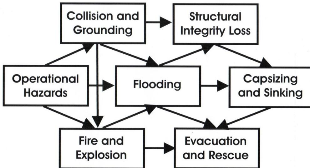
Fig. 8: Structure of Hazardous Scenarios in Ship Safety (adapted from Vassalos [62])
