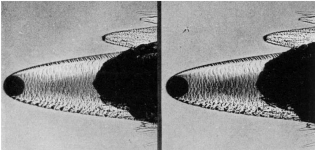
Fig. 10: Wolfgang Struth. Stereoscopic schlieren photograph of a shot into vapour of carbon tetrachloride. 1963. Source: Struth 1963: 446.
