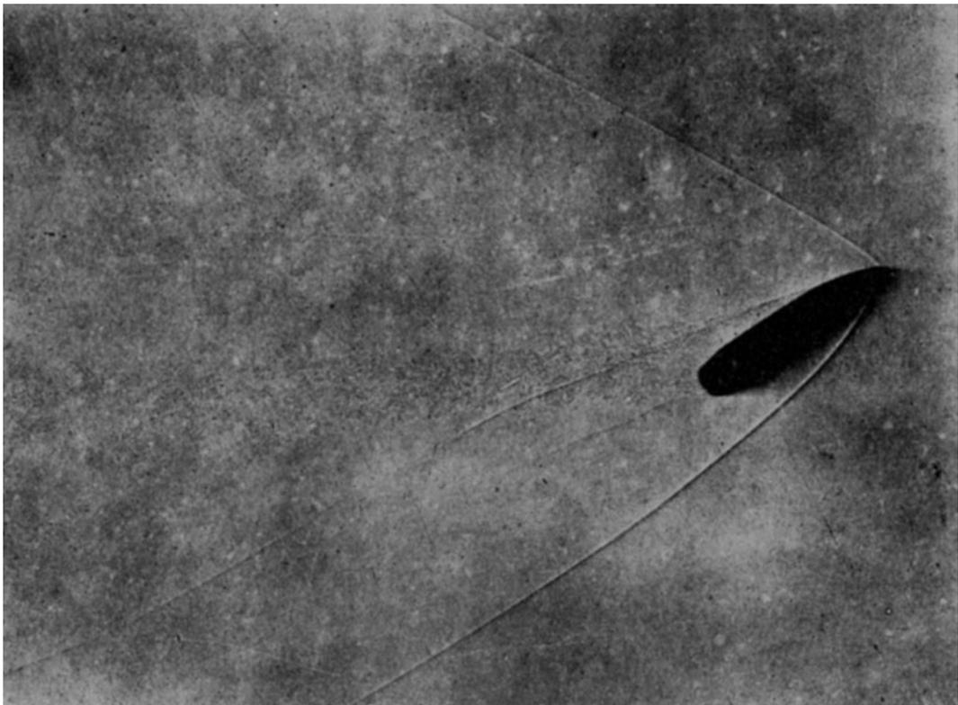
Fig. 4: Dayton C. Miller. Shadowgraph of a tumbling projectile. 1937. Source: Miller 1937: 82.
