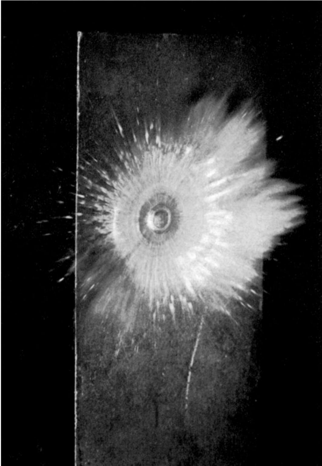
Fig. 5: Harold E. Edgerton. Front-lit photograph of a projectile's impact on a steel block. 1954.
