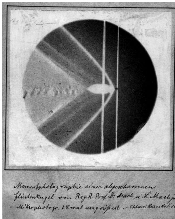
Fig. 2: Ernst and Ludwig Mach. Schlieren photograph. Negative. 1888-89. Source: Keller 2009: 231.
