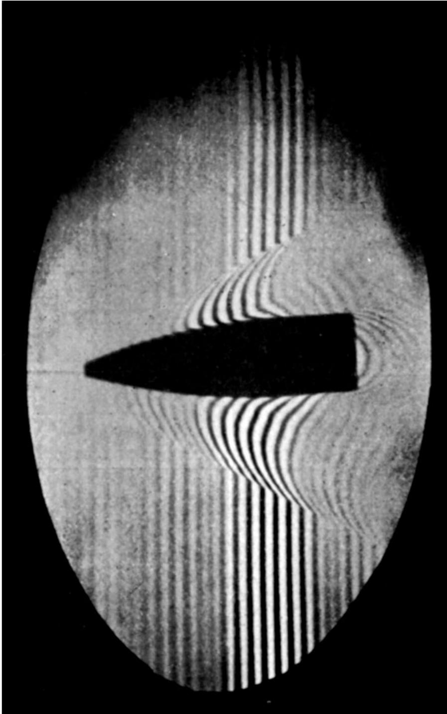
Fig. 3: Carl Cranz. Interferometric photograph. 1927. Source: Cranz 1927: 402.
