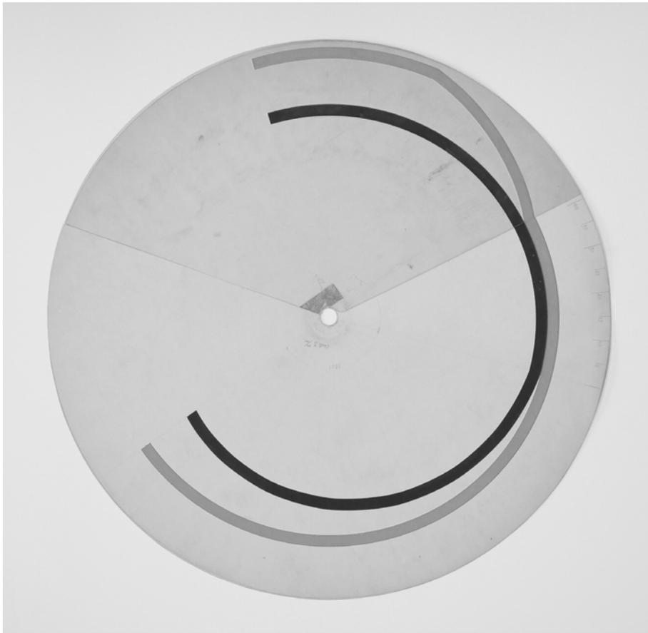
Fig. 7: Disc for the launching effect. This is the same pair of discs as in figure 6, but with a larger interval inserted, one which corresponds with  $42^\circ$ . At one rotation per second, this disc would have presented an interval of 114ms. Here the causal impression is about to disappear, and more than half of the subjects reported that they saw two separate events. From the Archive of the Laboratory of Experimental Psychology, Katholieke Universiteit Leuven (Photo Sigrid Leyssen).
