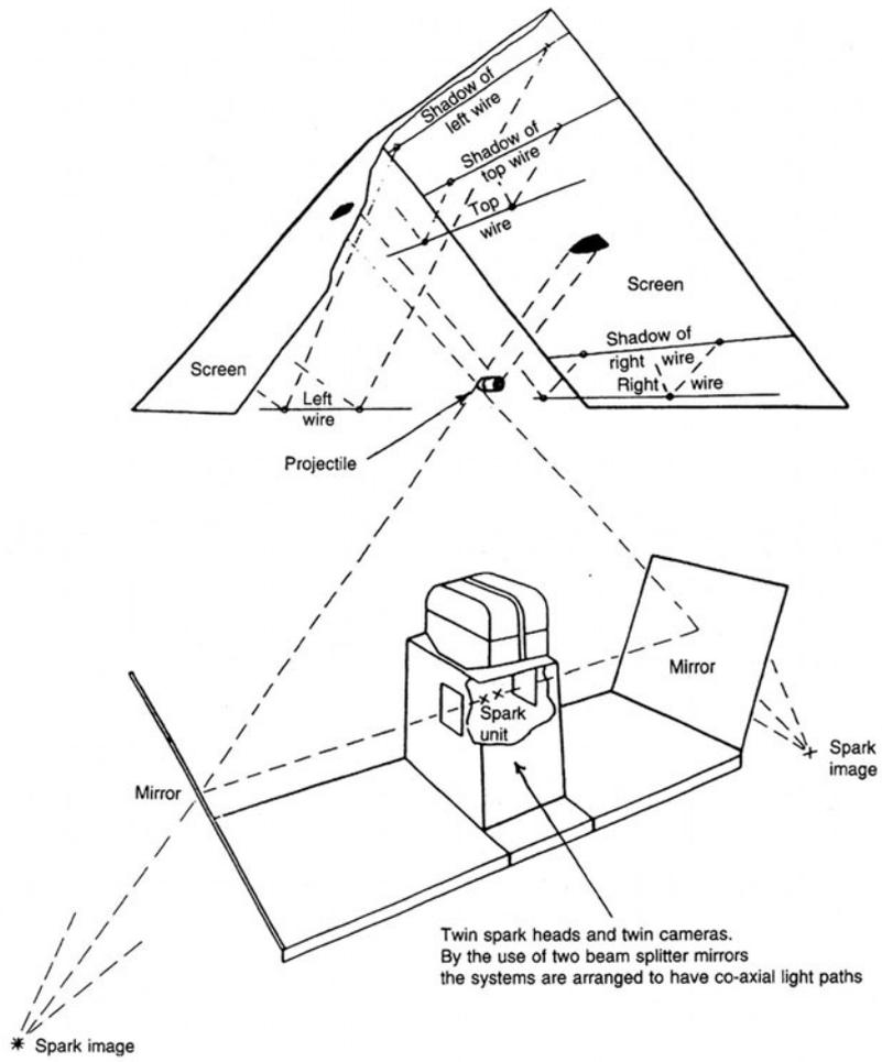
Fig. 6: Orthogonal photographic station in aeroballistic range. Source: Fuller 1997b: 225.
