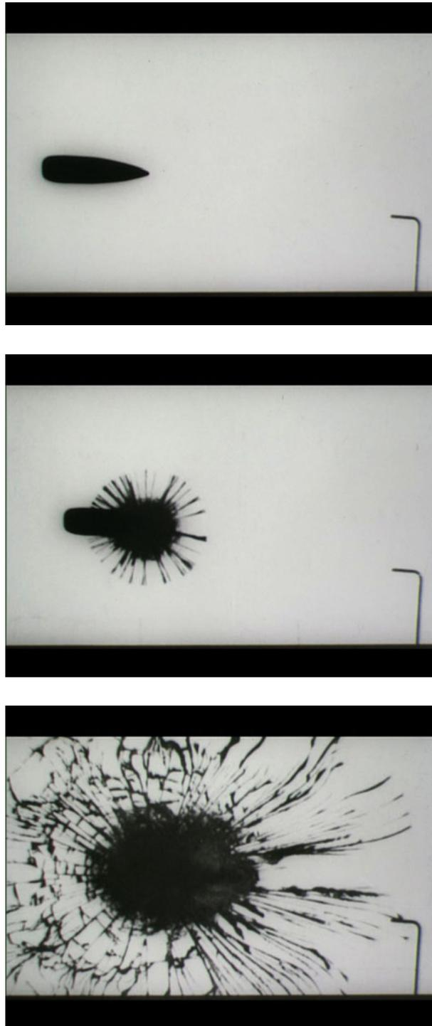
Fig. 26.1, 26.2, 26.3: Stills from a shot in Hubert Schardin, Wolfgang Struth and Dietrich Elle's film *Der Bruchvorgang im Glas* (1942-44), originally recorded at 200,000 pictures/s. Source: IWF Wissen und Medien, Göttingen.
