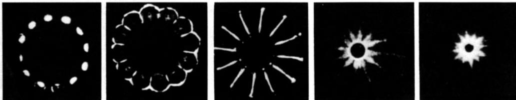
Fig. 15: Frames of an X-ray film showing a test implosion for the development of the denotator for the *Trinity* plutonium bomb. Manhattan Project. c. 1944-45. Source: Rhodes 1988: 821.
