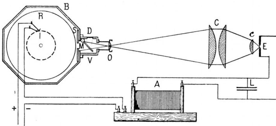
Fig. 7: Lucien G. Bull. Spark cinematograph. 1904. Source: Bull 1928: 143.
