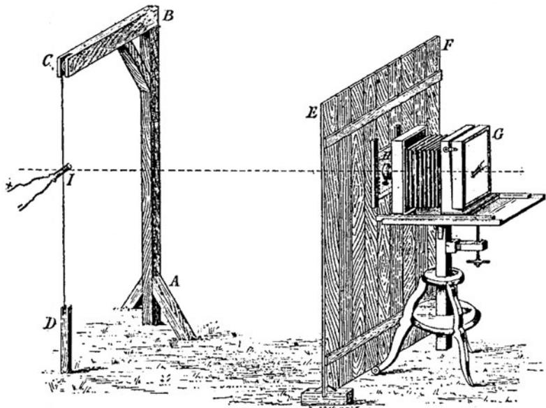
Fig. 17: Alfred Siersch. Protective wall for photographing small explosions. 1896. Source: Siersch 1895-96: 7.
