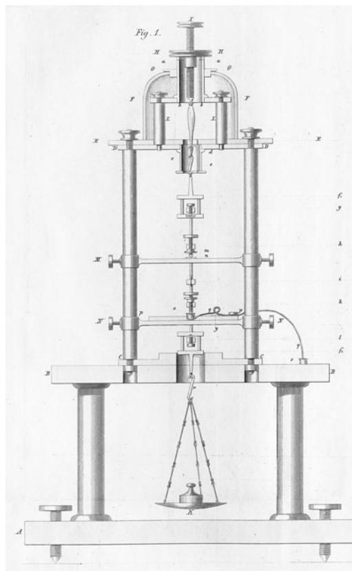
Fig. 2: Frog frame (1850). This half wooden, half metal frame allowed for hanging and stimulating nerve-muscle preparations. The preparation was fixed to the adjustable screw I and protected by means of a bell-jar. To the lower part of the muscle was fixed a device with multiple contacts and adjustable screws as well as a weight for tightening the muscle.
