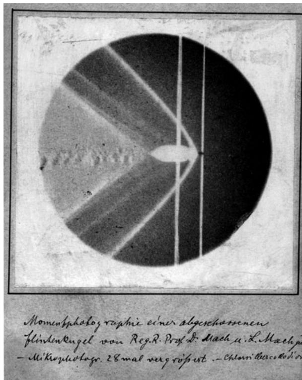
Fig. 2: Ernst and Ludwig Mach. Schlieren photograph. Negative. 1888-89. Source: Keller 2009: 231.
