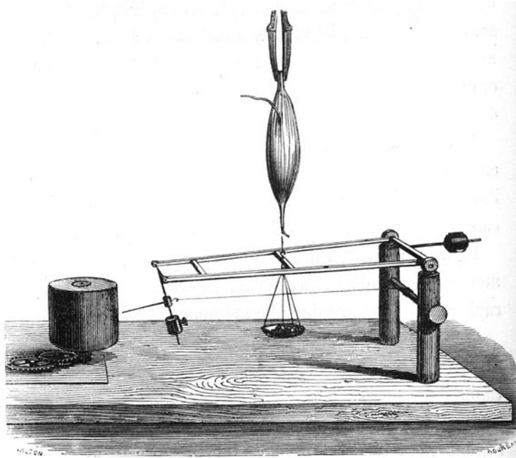
Fig. 6: Depiction of the »myograph« by Helmholtz according to Marey (1868). For the purpose of electric stimulation, a wire is inserted into a suspended frog muscle preparation. A metal frame and weight tightens the muscle. On the left side, a steel needle is attached to register muscle movements on the rotating glass cylinder. In comparison to Helmholtz's device, this myograph is a considerably simplified version of the instrument.
