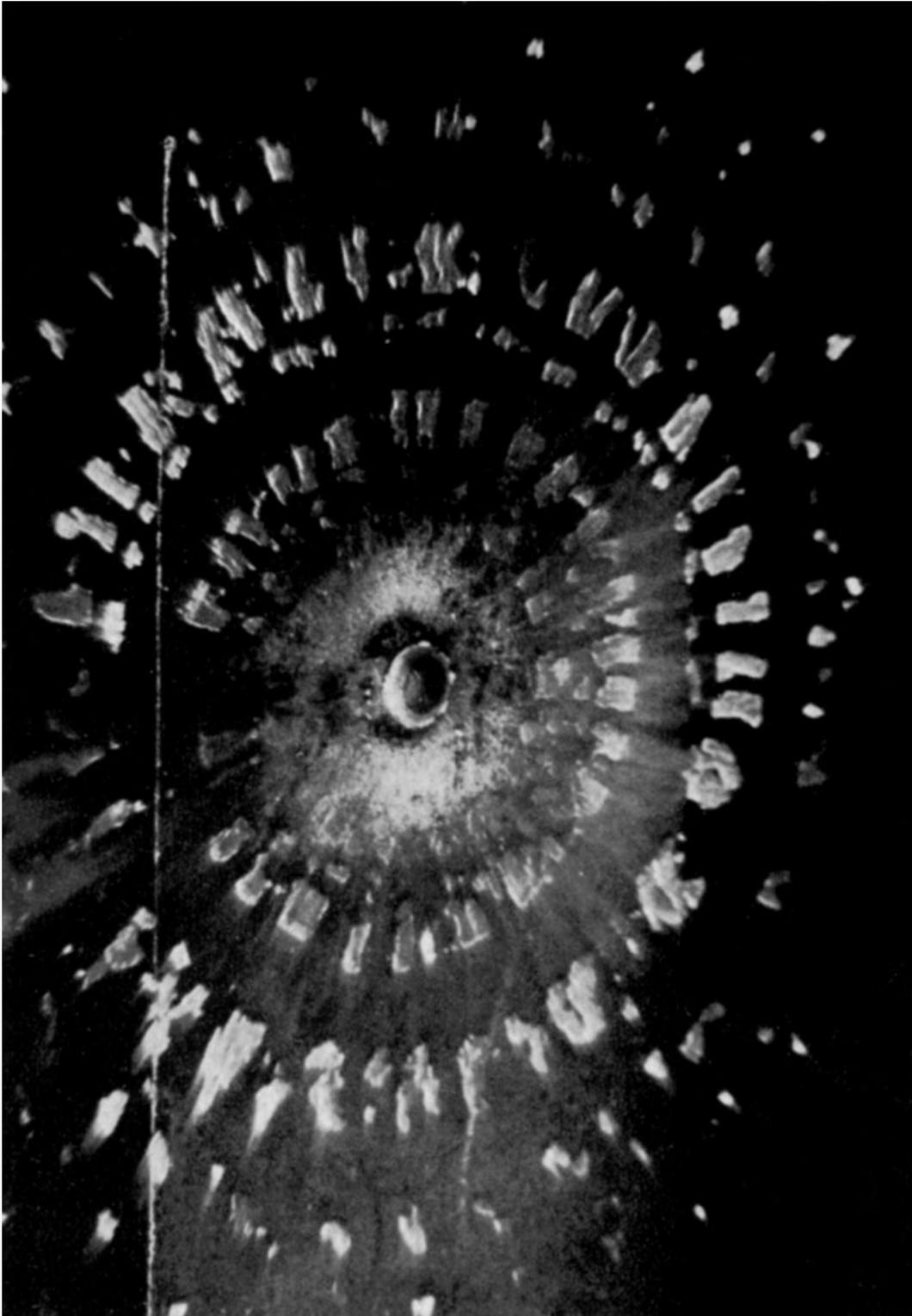
Fig. 23: Harold E. Edgerton. Photograph of the 'permanent splash' caused by a projectile's impact on a steel block. 1954. The picture belongs to the same sequence as the one reproduced in figure 5. Source: Edgerton/Killian 1954: 54.
