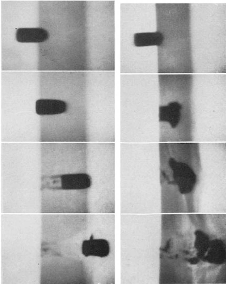
Fig. 14: Max Steenbeck. X-ray flash photographs of a lead projectile penetrating alder (left) and beech (right). 1938. Source: Steenbeck 1938: 476.
