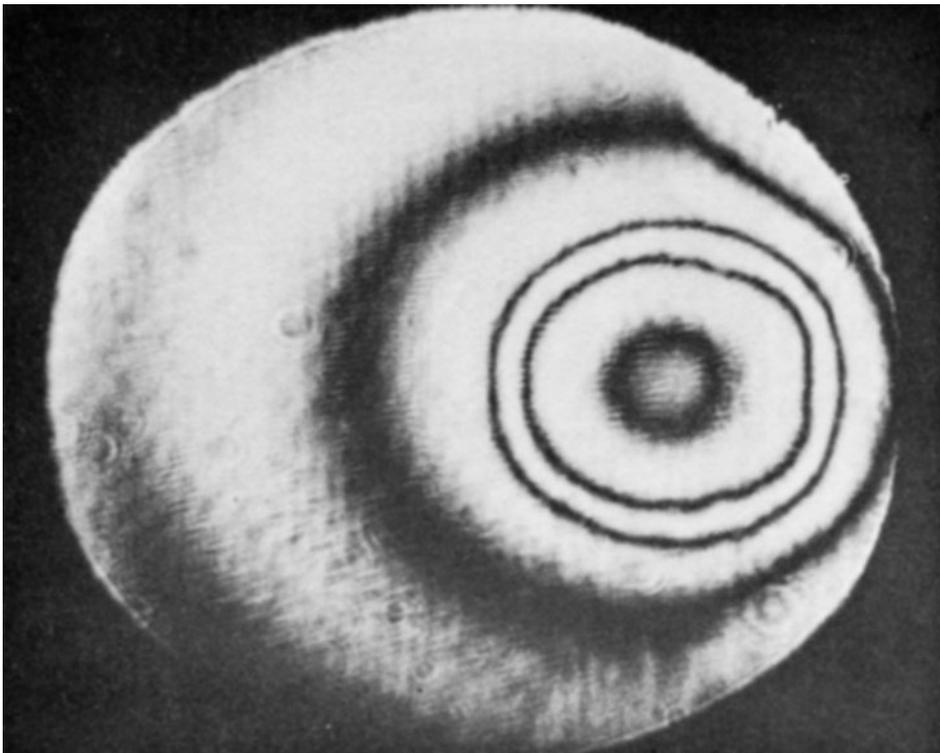
Fig. 16.1, 16.2: Paul Smigielski and Antoine Hirth. Photographs taken from reconstructed holographic interferograms of a shock wave generated by a laser, 5 and 20  $\mu$ s after initiation. 1970. Source: Smigielski/Hirth 1970: 323.
