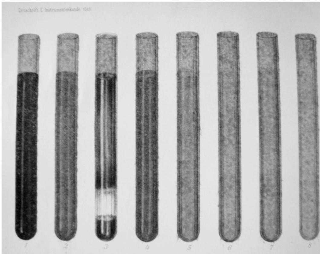
Figure 2: Glass testing with Iodine-Eosin Source: Mylius (1889), p. 52.
