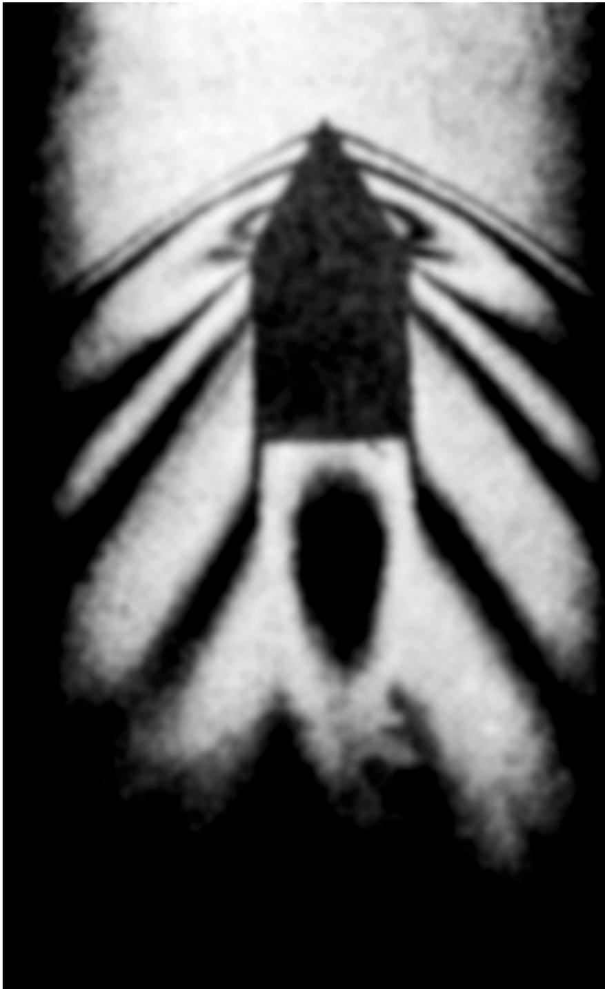
Fig. 13: Robert E. Brooks, Lee O. Heflinger and Ralph F. Wuerker. Photograph taken from a reconstructed holographic interferogram of a bullet moving through argon gas. Source: Brooks/Heflinger/Wuerker 1966: 646.
