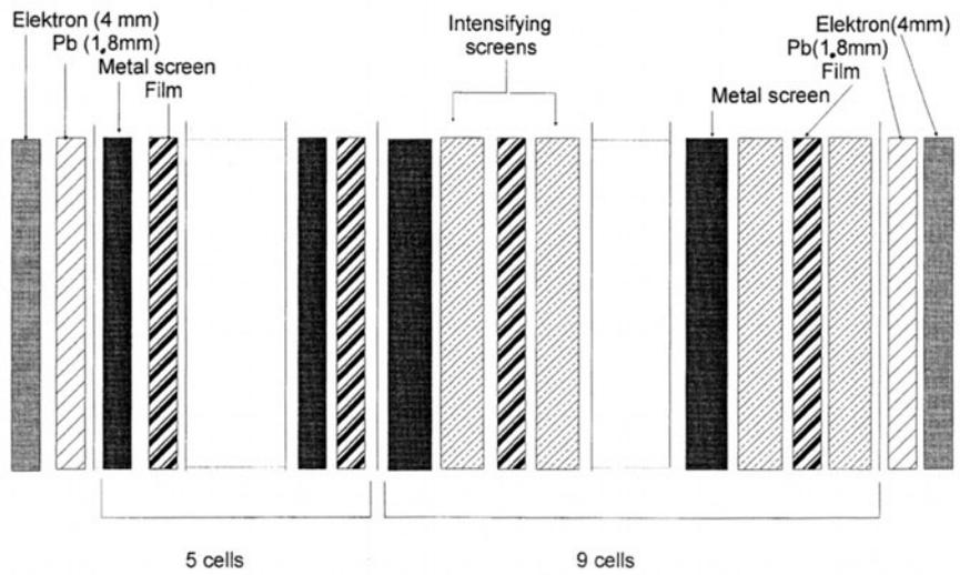
Fig. 19: Interior of cassette for X-ray film. Source: Cavailler 1997: 348.
