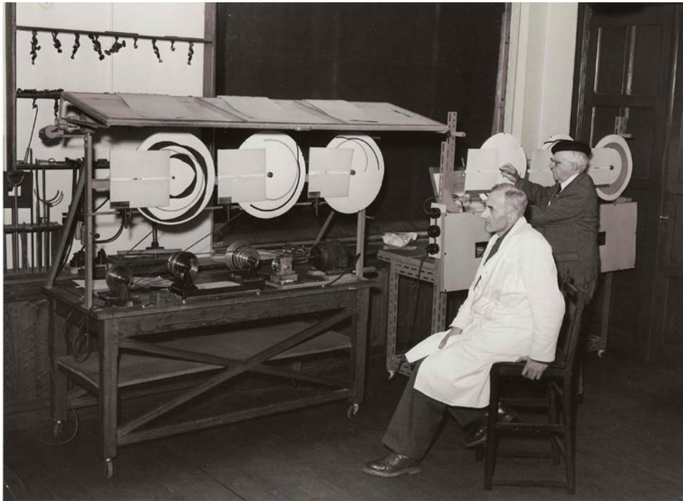
Fig. 3: The 'Banc Michotte', instrument used in the disc method in Michotte's experiments on perceived causality. In the back, Albert Michotte is arranging the discs, his colleague and former student Gérard de Montpellier is seated in front. Photograph from the Collection of the Library of the Faculteit Psychologie en Pedagogische Wetenschappen, Katholieke Universiteit Leuven, Leuven, Belgium.
