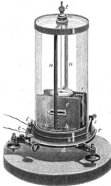
Fig. 3: Galvanometer according to du Bois-Reymond for electro-physiological precision measurements. Crucial components are a coil with windings of copper wire (a, b, c, e) and a magnetic needle suspended by means of a silk thread. Helmholtz used a similar device in his time experiments. It is unclear, however, whether he bought or constructed it.
