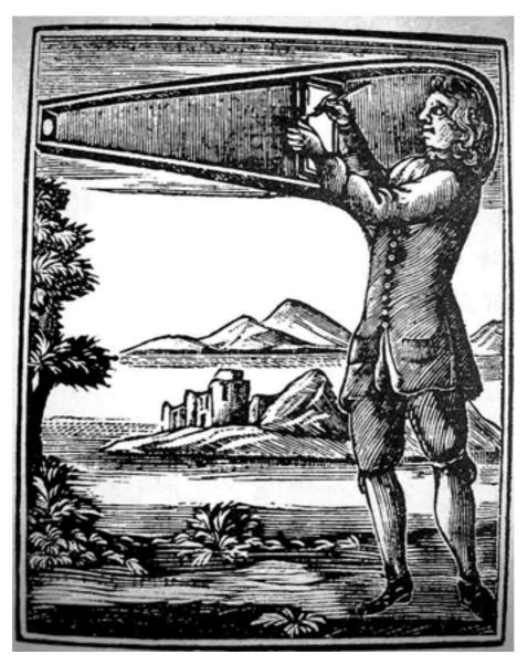
Fig. 8: Robert Hooke, Picture Box, 1694, image from Robert Hooke. "An Instrument of Use to take the Draught, or Picture of any Thing. Communicated by Dr. Hook [sic] to the Royal Society Dec. 19., 1694", in William Derham, Philosophical Experiments and Observations of the late eminent Dr. Hooke (London, 1726) 295.
