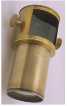
Fig. 9 B: Revolving turret for tent-type Camera Obscura, 1865, brass and glass, ca 7 x ca 3.5 in. (ca 18 cm x ca 9 cm). Physics Laboratory & Museum of Scientific Instruments, University of Urbino (photograph ©Physics Laboratory & Museum of Scientific Instruments, University of Urbino).
