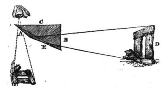
Fig. 20: Anonymous, Optical Principle of the Wollaston Camera Lucida, 1840, image in The Magazine of Science and School of Arts I, XLIII (1840): 338.
